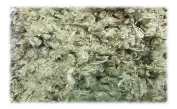
SRWF Granulated Wool – Cryogenic Rockwool
