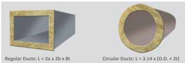
Regular Ducts: L = 2a \times 2b \times 8t
